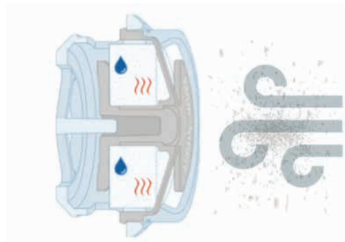
Figure 4. HME internal structure aids in filtering air, warming air, and protecting against environmental pollutants/particles
