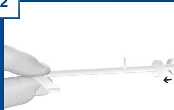
Place the tip of the inserter tool into the open end of the plug insert.
